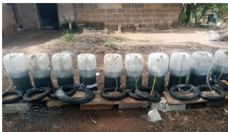
Figure 2. Anaerobic digestion set-up outside the lab.
