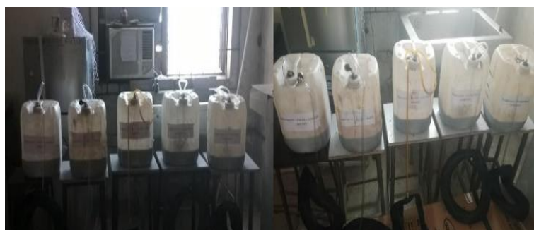
Figure 1. Anaerobic digestion set-up inside the lab.
