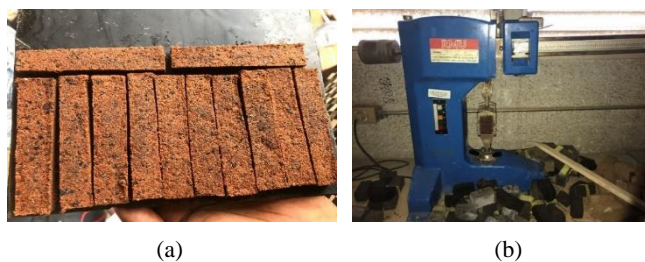
Figure 2. (a) Flexural test samples (b) Automatic flexural testing machine.
