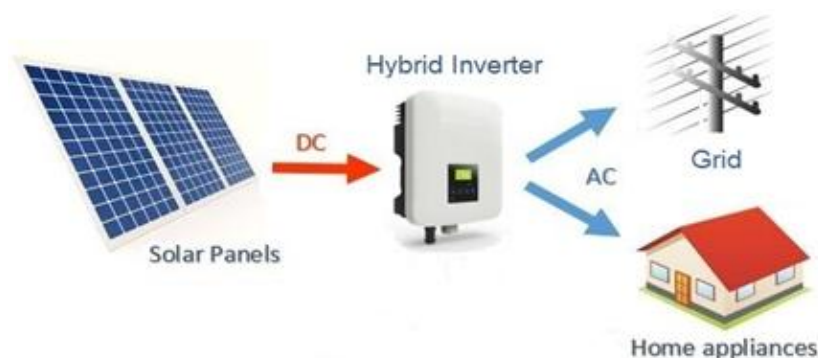
Figure 2. House solar system integrated with the local microgrid.
