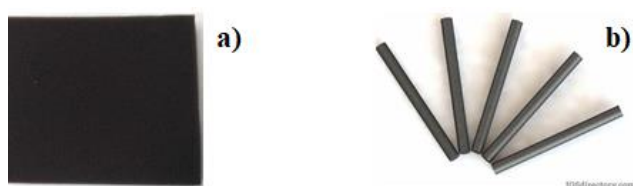
Figure 2. a) Carbon foam electrode, b) Graphite rod electrode.
