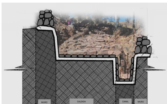
Figure 17. Road section delimited by walls Segment 2. Source: ATLAS Consulting Project - Adjustment Annex 18-2019.
