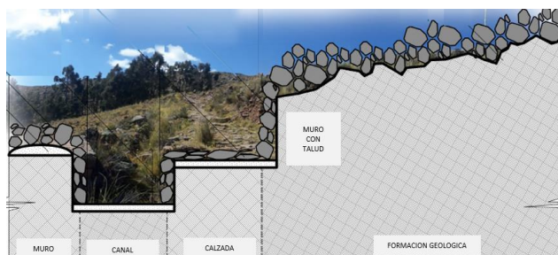
Figure 20. Road section with slope cut. Source: ATLAS Consulting Project - Adjustment Annex 18-2019.
