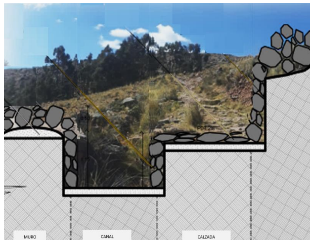
Figure 25. Path with draining channel section. Source: ATLAS Consulting Project - Adjustment Annex 18-2019.
