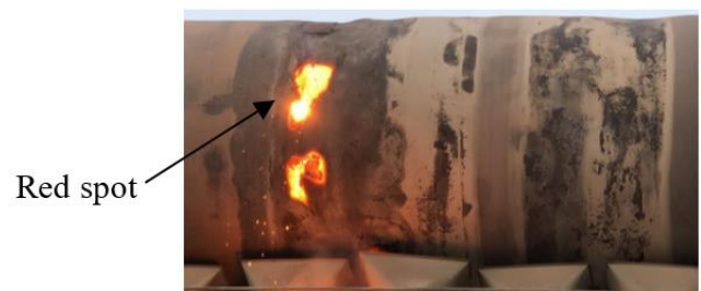
Figure 2. Refractory failure that created a red spot on the kiln shell.
