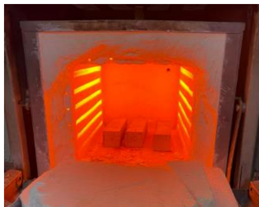
Figure 5. Sample in a muffle furnace for CCS testing.
