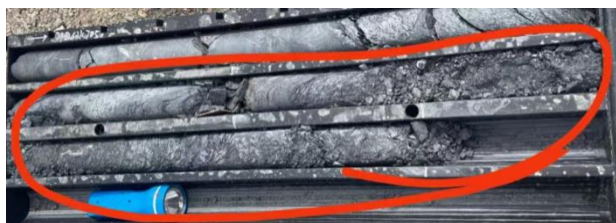
Figure 5. Coring of potassium-based film-forming drilling fluid used in field.
