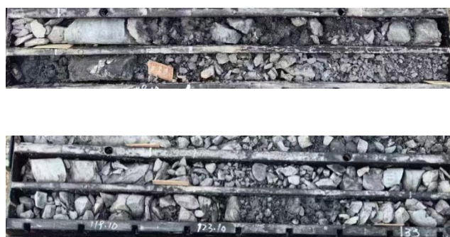
Figure 3. Core taken in situ with original bentonite polymer.
