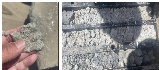
Figure 2. Loose, broken core retrieved from field.
