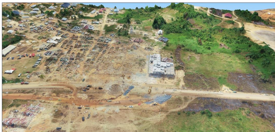
Figure 9. 3D model of Appiatse Community showing the crater and the entire destruction caused by the blast incident.
