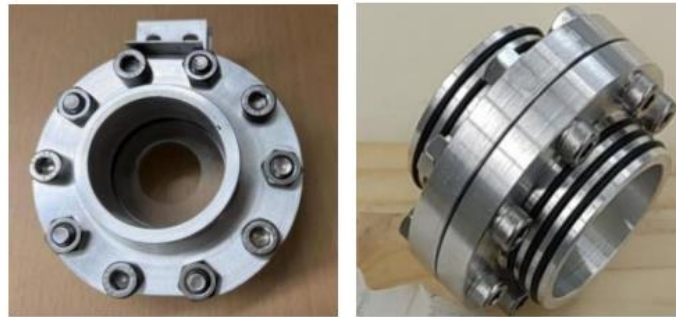
(c) Mass block with hermetic seal
