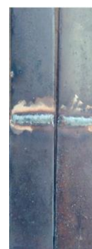
Figure 3. Specimen after welding.
