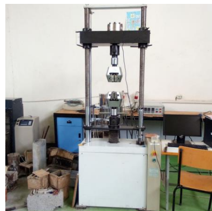
Figure 7. (right) Tensile testing machine.
