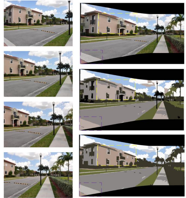
Figure 2. The images, stitched Image, the semantic segmentation result of stitched image using the method designed by Asako Kanezaki, and the semantic segmentation result of stitched image using the method designed by Asako Kanezaki combined with the IDCM.
