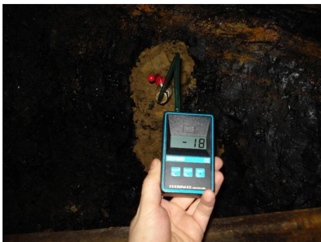
Figure 5. Pressure measurement in the sampling well.
