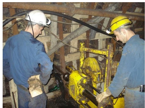
Figure 2. Coal sampling from a isolation wall by coring.
