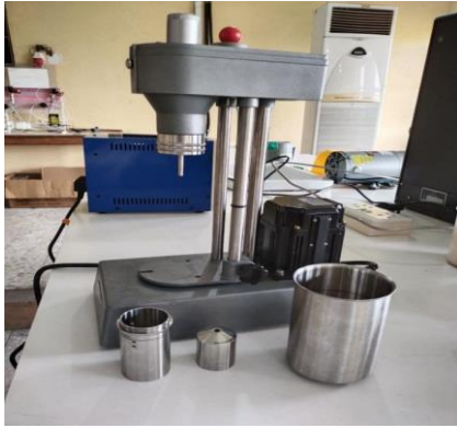
Figure 11. Fann V-G viscometer.
