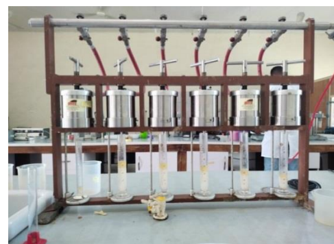
Figure 12. Ofite filter press stack.
