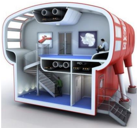
Figure 4. Cross-section, elevated living and research wings of the Juan Carlos I, Antarctic Research Station. Designed by Hugh Broughton Architects, & ARC. Source: https://spacearchitecture.org/portfolio-item/juan-carlos-1-antarctic-base/ . [27].
