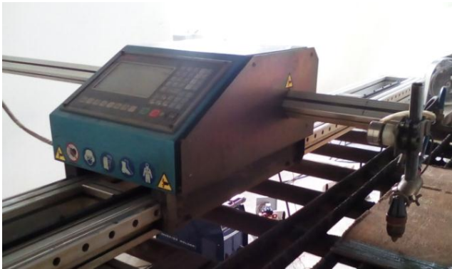
Figure 6. CNC plasma cutter and test place.
