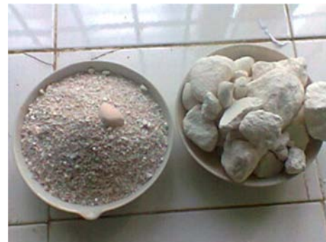
Figure 3. Non-Calcinated Ikare Clay Sample.
