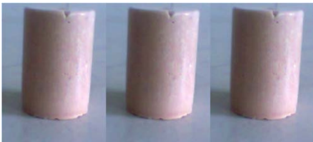
Figure 6. Geopolymer Samples synthesized from Ikare Kaolinite.
