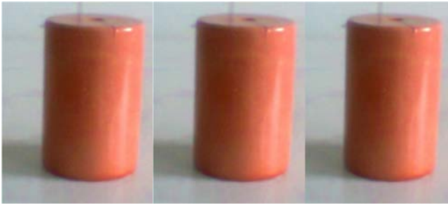
Figure 5. Geopolymer Samples synthesized from Ikere Kaolinite.
