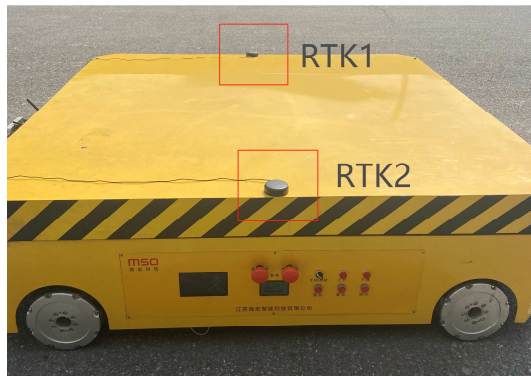
Figure 4. Diagram of the actual RTK installation.
