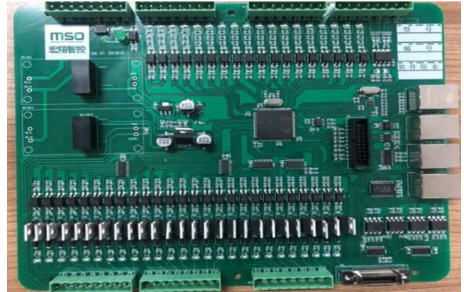
Figure 3. Lower computer of multi-shaft controller.
