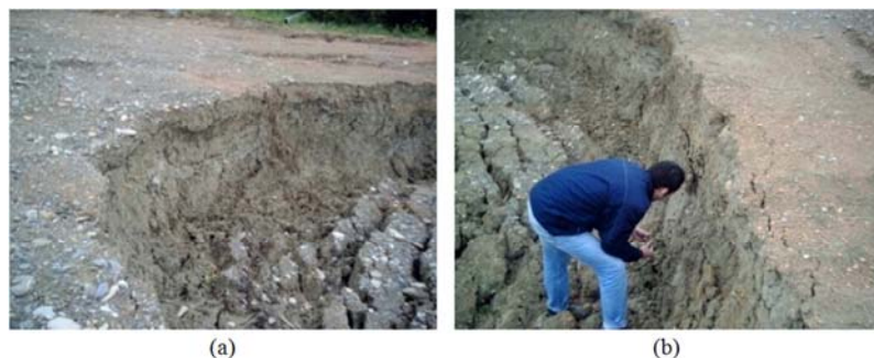
Figure 13. Two rotation landslides on the marl-filled layers.
