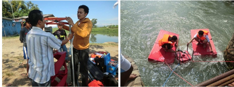
Figure 8. VATT Gorlov assembly (left) and experimental (right).
