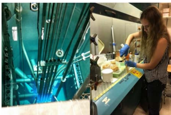
Figure 3. Neutron irradiation at the PULSTAR reactor (left: reactor core and irradiation tubes at the PULSTAR reactor; right: a student worked by the hot cell to unpack the samples after irradiation of short-lived isotopes).
