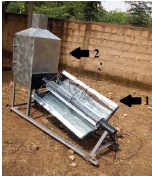
Figure 1. Picture of the solar dryer [13].
