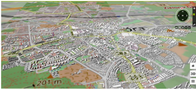
Figure 4. Model of the City of Zielona Góra, created in CityGML standard, level of details (LOD1), viewed in virtualcitySUITE, 2018.
