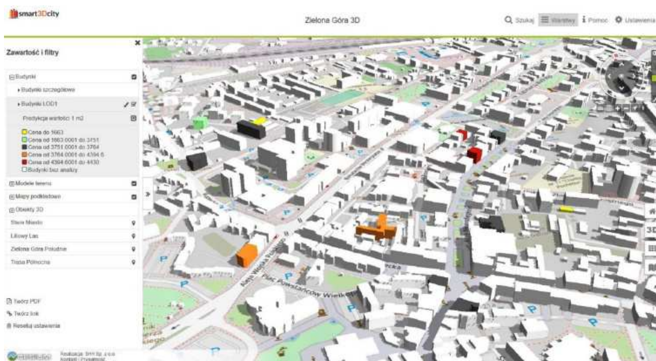
Figure 6. Resulting model of generation of buildings of the City of Zielona Góra in CityGML LOD1, presented in virtualcitySUITE software, with the result of deep learning of neural networks, in the area of prediction of price of 1m 2 of real estate.
