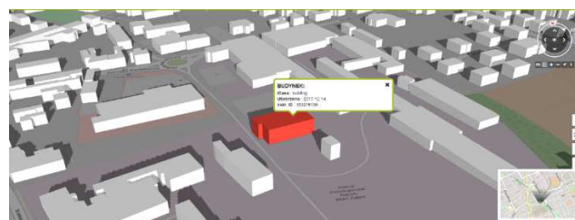
Figure 3. The geometry of an example building with the basic descriptive parameter, created in CityGML standard, level of details (LOD1), viewed in virtualcitySUITE, 2018.
