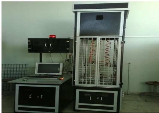
*Figure 9. Impact test machine.*
