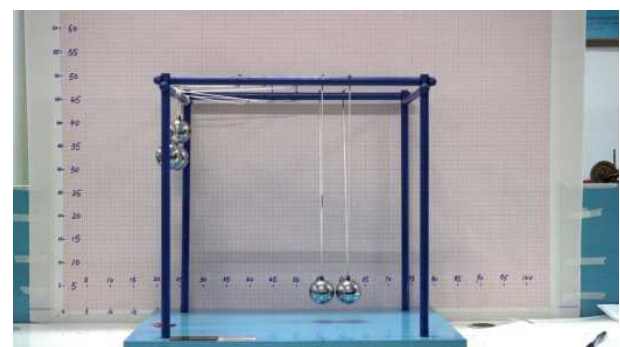
Figure 8. The experiment of Newton's Cradle of 2 balls.
